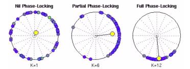
Nil, partial and full phase-locking in an all-to-all network of Kuramoto oscillators. Phase-locking is governed by the coupling strength K and the distribution of intrinisic frequencies  $\omega$ . Here, the intrinsic frequencies were drawn from a normal distribution (M=0.5Hz, SD=0.5Hz). The yellow disk marks the phase centroid. Its radius is a measure of coherence.
