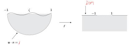
We want to compute and control the oscillations frequencies of the free surface, in a bounded container. We put ourselves in the frame of an incompressible, non viscous fluid (water), in contact with solid walls.
